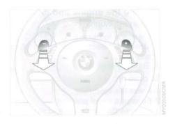
Changing gear via the rocker switches on the steering wheel:
